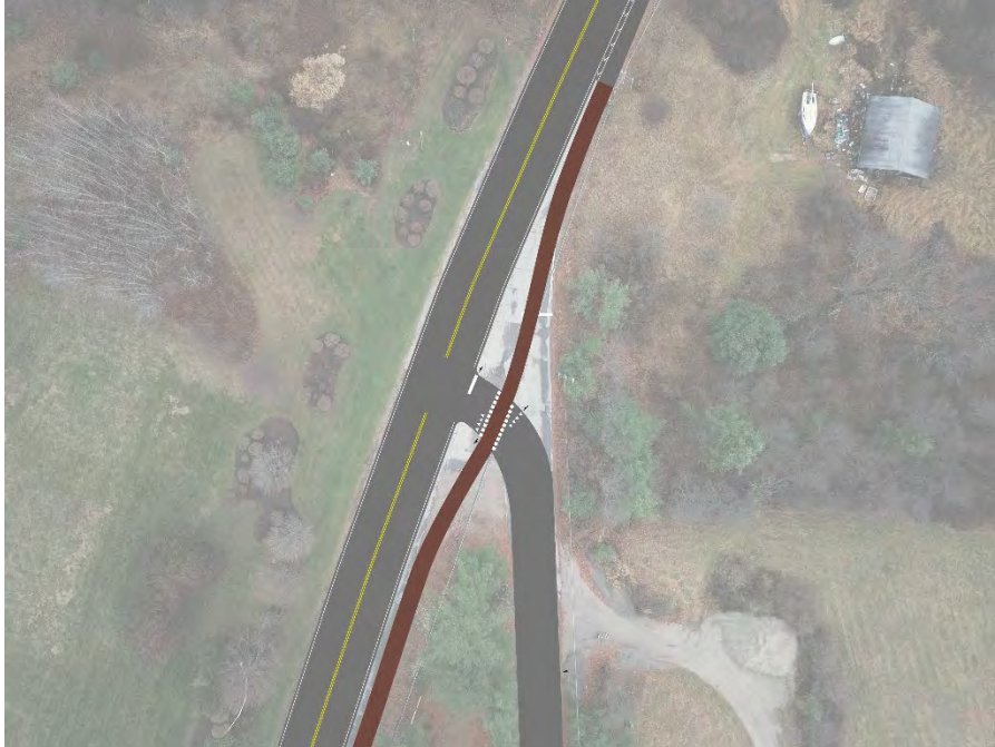
Figure 13 Graphical depiction of a restructured intersection at Amherst Street and Border Street. A transition from sidepath to on-road treatment can also be found at the top of this picture.
