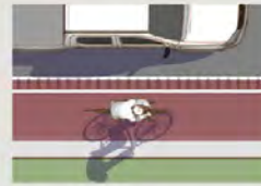
A narrow buffer space—two normal 4" solid white lines separated by an 18" or greater space.
