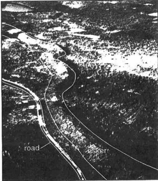
Figure 9. Aerial photograph taken in the 1940's of the Pine River Esker in Ossipee, east-central New Hampshire. Sand and gravel from this esker was used to build the road seen next to the esker in the photograph. Since the photograph was taken, much of the Pine River Esker has been mined for large construction projects. (From Goldthwait and others, 1951, fig. 20.)
