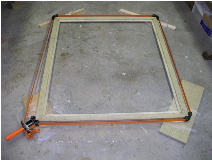
Photo 2-8: Mitered corners clamped with a web corner clamp
